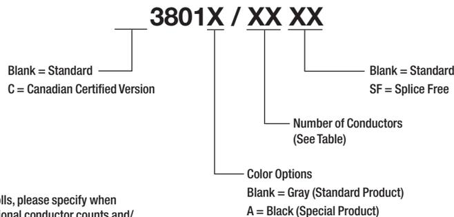
Note: Available in standard 100 ft or 300 ft rolls, please specify when ordering. Contact 3M for availability of additional conductor counts and/or custom roll lengths.
