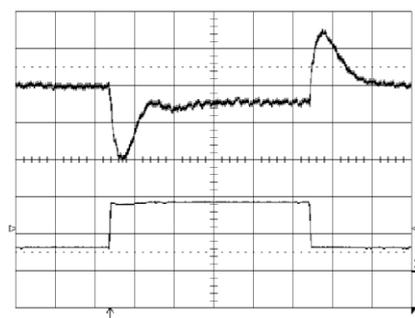
Output voltage response to load current step-change (0.3-0.9-0.3 A) at:
