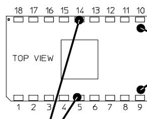
Pin 5 of pin 14 for measurement of minimum pin (solder joint) temperature,  $T_{PIN}$
