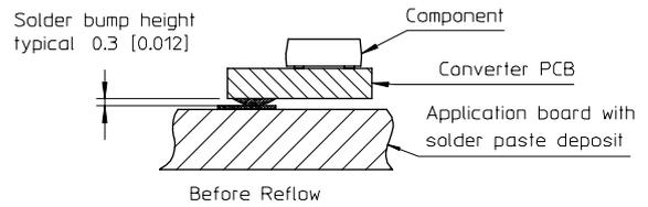
Solder joint thickness: 0.1 to 0.3 [0.004 to 0.012]
