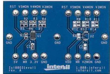
FIGURE 4. ISL88031EVAL1 SCHEMATIC AND PHOTOGRAPH
