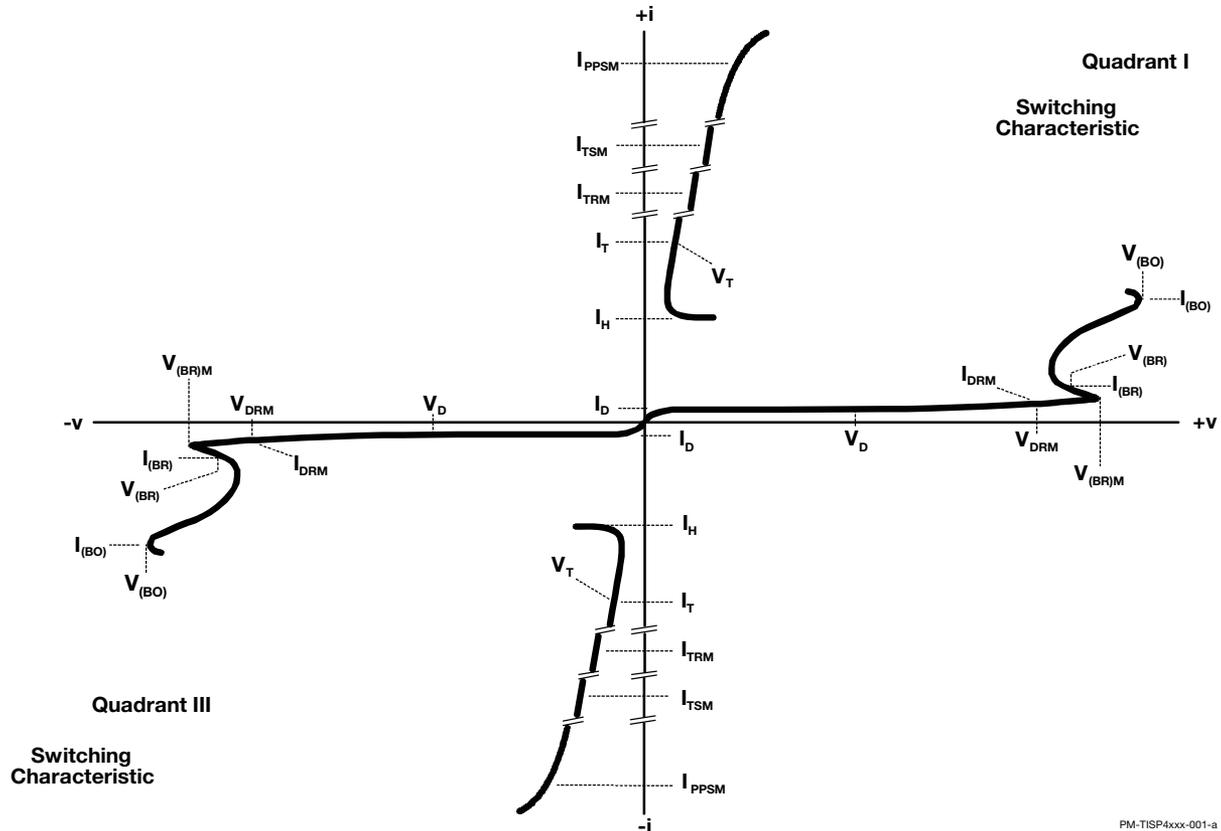
Figure 1. Voltage-Current Characteristic for Tip and Ring Terminals
