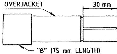
Slide 'B' (75mm length) onto the tape.
