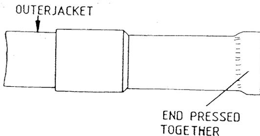
Use the hot air gun to gradually shrink into position. This is achieved by playing the hot air gun over the periphery of 'B'.
