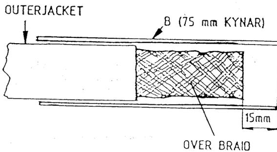
Slide 'B' over the end of the tape so that it overhangs the end by approx. 15mm.
