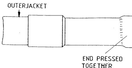
Use the hot air gun to gradually shrink into position.
