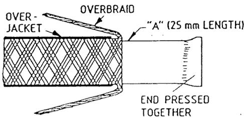
Place 'A' (25mm length) over the exposed inner jacket so that it rests next to the braid and overhangs the end of the tape.
