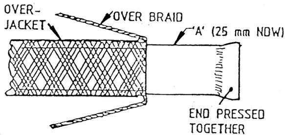
Un-ravel the over braid, folding the strands back over onto the overjacket.
