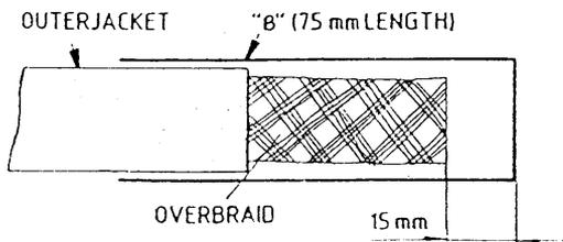
Slide 'B' over the end of the tape so that it overhangs the end by approx. 15mm.
