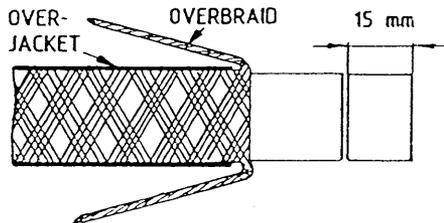
Loosen the overbraid folding the strands over onto the overjacket.
