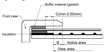
10.2.3 The corners of the product are not tipped when installing to case, so, we suggest that the corner may be designed R part of case so as not to apply load to corner of touch panel.
