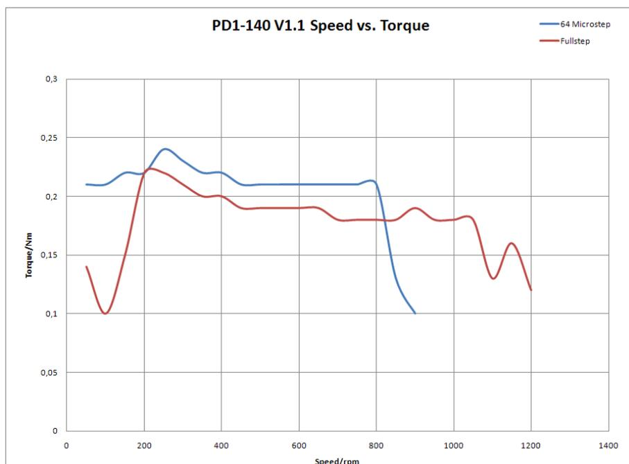
Figure 7.1: PD1-140-42-SE torque curve
