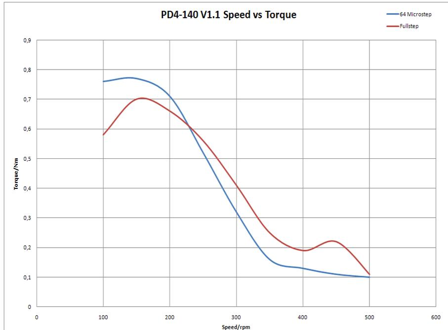
Figure 7.4: PD4-140-42-SE torque curve
