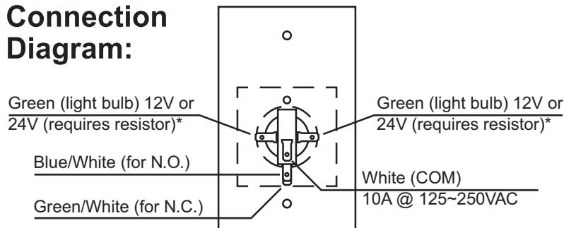
\*Note: Use 150 ohm, 1 watt resistor on either one of Green wires for 24 volt bulb operation.
