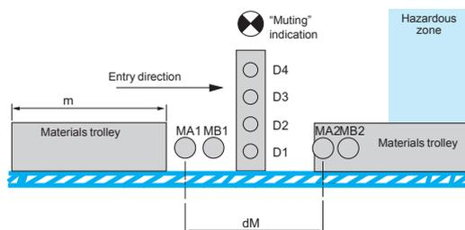
D1, D2, D3, D4: monitoring photo-electric sensors.
