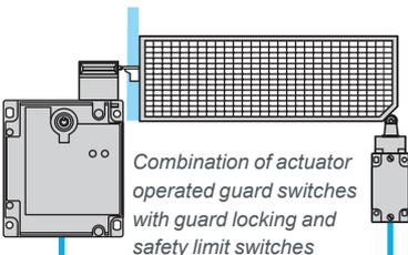
Combination of actuator operated guard switches with guard locking and safety limit switches
