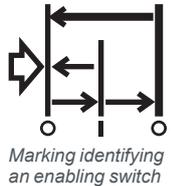
Marking identifying an enabling switch
