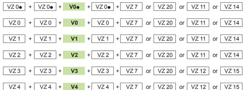
**Note :** The add-on modules mounted next to the switch body are main pole modules. Maximum of 3 main pole modules per switch body.
