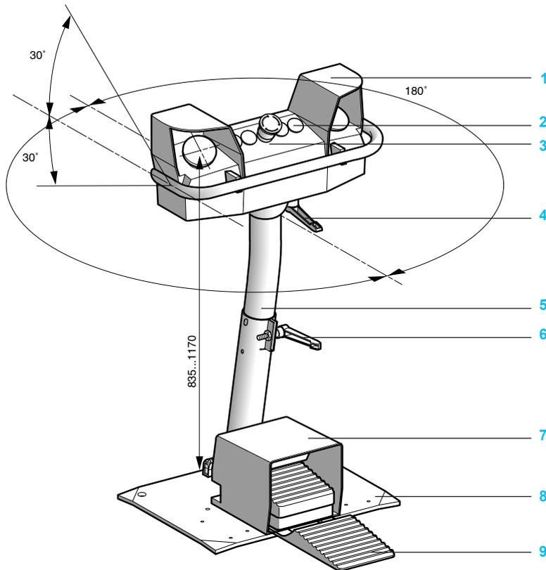
The control station **1** has five cut-outs ( $\varnothing 22$  mm) **2** as standard. Five additional cut-outs are possible **3**. Its pedestal **5** enables the following quick and simple adjustments:
