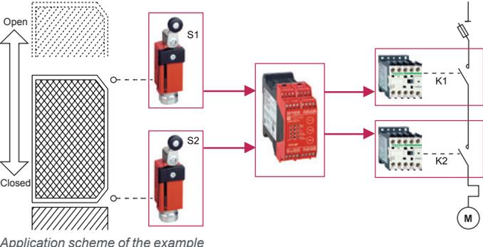
The process suggested by the standard is iterative and a few estimations are therefore necessary in order to obtain the expected result. In view of the required performance level, we have chosen a solution with redundant circuit.
