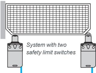
System with two safety limit switches
