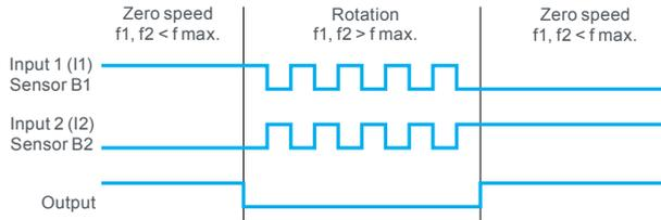
The two sensors to be arranged that only one sensor is activated at any given time. If the inputs are in the low state, the zero speed signal will disappear after  $t=1/f$  seconds and an open-circuit will be indicated. If the 2 inputs are in the high state, the zero speed signal will disappear after  $t=1/f$  seconds and a short-circuit will be indicated. If the 2 inputs are in the high or low state after starting, no enabling will take place.
