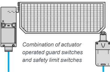
Combination of actuator operated guard switches and safety limit switches
