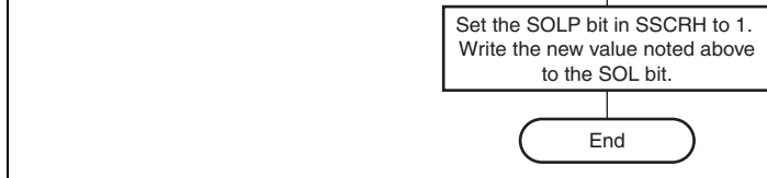
Figure 16.14 Procedures when Changing Output Level of Serial Data
