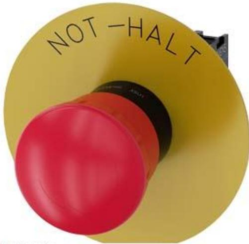
EM. STOP MUSHROOM PUSHBUTTON, 22MM, ROUND, PLASTIC, RED, 40MM, LATCHING, POSITIVE LATCHING, ROTATE TO UNLATCH, WITH YELLOW BACKING PLATE, INSCRIPTION: NOT-HALT, WITH HOLDER, 1NC, SCREW TERMINAL
