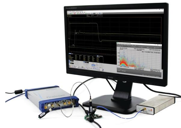
Standard connectorized SMA, PC3.5 and K accessories such as attenuators, signal dividers, multiplexers, filters and cables of varying length and performance can also be placed in series with the probe output to further condition or route the signal.
