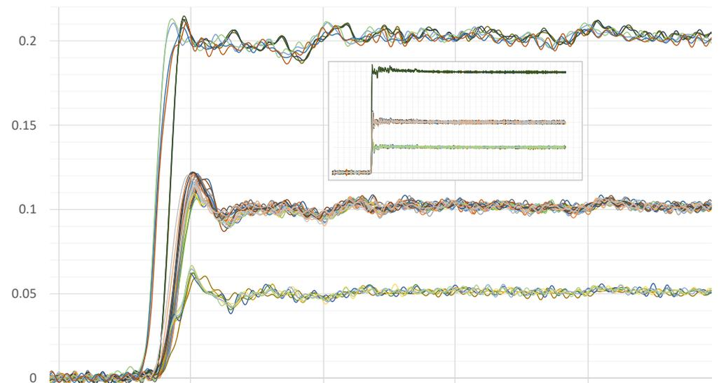
PicoConnect passive probe family pulse shapes – first 2 ns (inset 17 ns)
