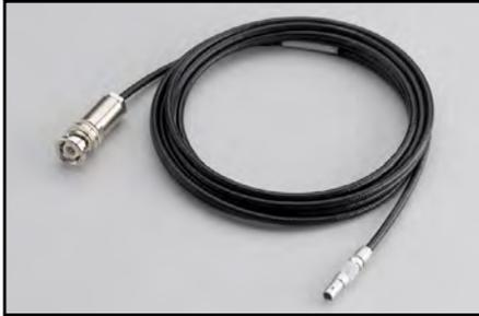
**Model 4200-MTRX\*:** Ultra low noise SMU triax cable is terminated with a miniature male triax connector on one end and a standard 3-slot male triax connector on the other. This cable connects a Model 4200-SMU or 4210-SMU source measurement unit installed in a Model 4200-SCS to a test fixture. (4200-MTRX\* cables are intended only for connection to an SMU that does not have a 4200-PA PreAmp installed.)
