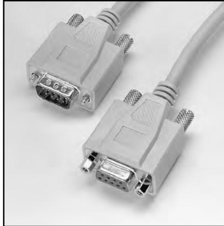
**Model 7009-5 Shielded RS-232 Cable:** 1.5m (5 ft) RS-232 cable with a male DB-9 connector at one end and a female DB-9 connector on the other end. Wired as a straight through, not as a null modem cable.
