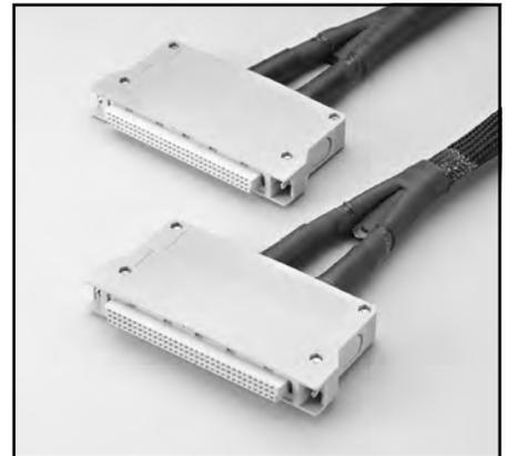
**Model 7020-MTC-2:** 2m (6.6 ft) mass terminated cable assembly for connection to 7020. The cable has 45 pairs with outer shield. The cable is terminated at each end with 96-pin female DIN connectors with strain relief.
