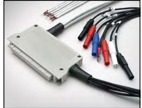
**Model 7019C-MTCI-2 6-wire Kelvin Extender and Instrument Cable:** Used with Model 7019-C 6-Wire Ohms Matrix Card and a SourceMeter SMU instrument. The SourceMeter cables are 0.6m (2 ft) long and the DUT cables are 2m (6.6 ft) long. The cable set is used in a basic system to test a resistor network.
