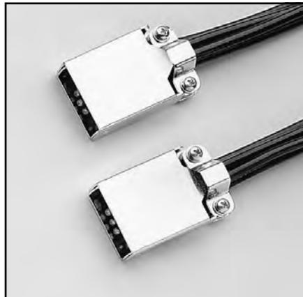
**Model 7152-MTC-\*:** Five low noise triax cables terminated in 6-position M-series coax connector blocks. Provides quick connection between 7152 matrix cards and is compatible with Model 7152-MTR connector. Also available in 3m (10 ft) length for connection between the matrix and the device under test.
