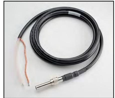
**Model 2290-10-SHVUC:** 3m (10 ft) of RG-213/U coaxial cable terminated with a SHV male connector on one end and unterminated cable on the other end. Maximum operating voltage is 10,000Vrms.
