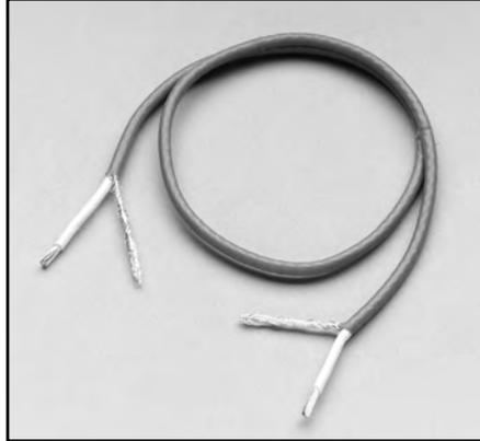
**SC-182:** Low inductance ( $42\text{nH/ft}$ ) coaxial cable for minimizing test lead impedance in circuits using fast transient response power supplies. The cable is sold by the foot and comes without connectors.
