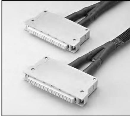
**Model 7035-MTC-2:** 2m (6.6 ft) mass terminated cable assembly for connection to 7035. The cable has 45 pairs with outer shield. The cable is terminated at each end with 96-pin female DIN connectors with strain relief.
