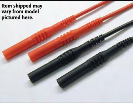
**Model 8607 1kV Source Banana Cable Set:** The 8607 cable set is made up of one red and one black high voltage test lead with fixed safety banana plug ends. The leads are 1 meter (3.3 ft) long and have a voltage rating of 1500V DC.
