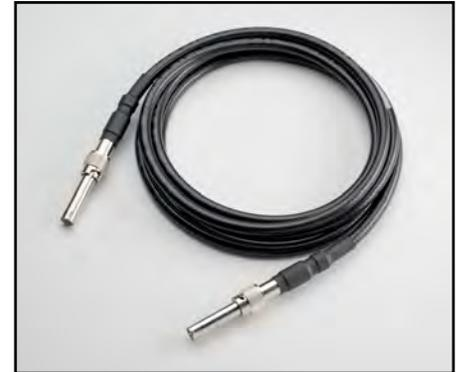
**Model 2290-10-SHV:** 3m (10 ft) of RG-213/U coaxial cable terminated with a SHV male connector on both ends. Maximum operating voltage is 10,000Vrms.
