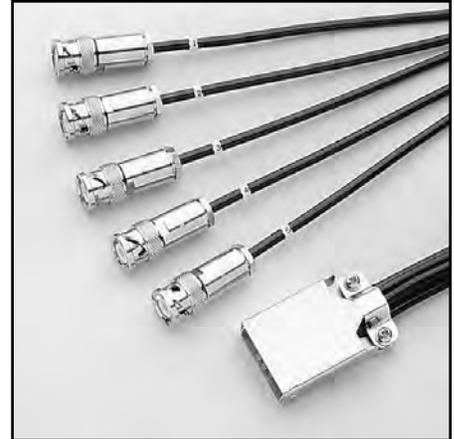
**Model 7152-TRX-10:** Set of five 3m (10 ft) low noise triax cables terminated at one end in a single M-series connector block and at the other end in 3-slot triax connectors. This cable is most useful for direct connection to electrometers and Source/Measure Units.
