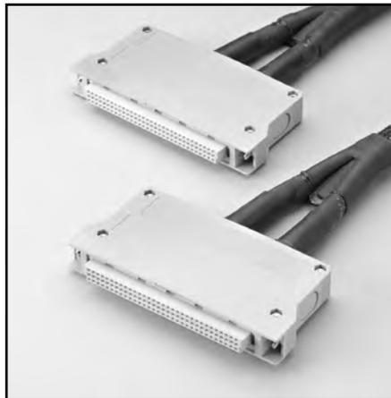
**Model 7011-MTC-x:** Mass terminated cable assembly for connection to 7011-C and other switching cards. The cable has 45 pairs with outer shield. The cable is terminated at each end with 96-pin female DIN connectors with strain relief.
