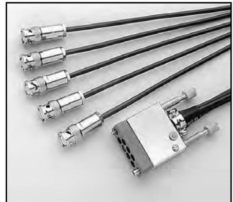
**Model 7153-TRX:** 2m (6.6 ft) low noise cable assembly with M-series connector at one end for row or column connections to the 7153, and five 3-slot male triax connectors at the other end. Two 7153-TRX cable assemblies are required to make all connections to the 7153 card.
