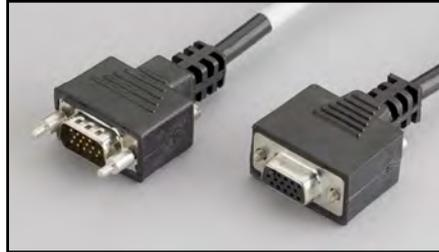
**Model 4200-RPC\*:** Remote PreAmp cable terminated at each end with a high density DB15 connector. This cable connects a Model 4200-SMU or 4210-SMU source measurement unit installed in a Model 4200-SCS to a remotely mounted Model 4200-PA PreAmp.
