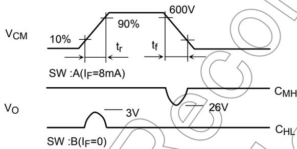
$$C_{ML} = \frac{480 \text{ (V)}}{t_r \text{ (\mu s)}}$$
