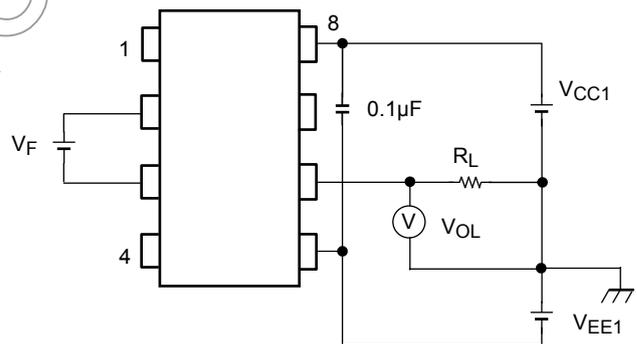
Test Circuit 5:  $t_{pLH}$ ,  $t_{pHL}$ ,  $t_r$ ,  $t_f$
