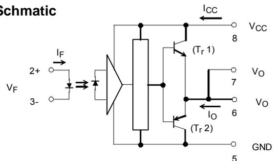
A 0.1 $\mu\text{F}$  bypass capacitor must be connected between pin 8 and 5 (See Note 5).
