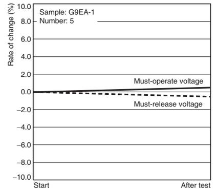
Characteristics were measured after applying a shock of 490 m/s to the test piece 3 times each in 6 directions along 3 axes. The percentage rate of change is the average value for all of the samples.
