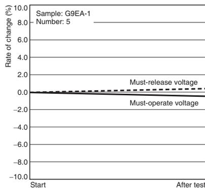
Characteristics were measured after applying vibration at a frequency of 10 to 55 Hz (single amplitude of 0.75 mm) to the test piece (not energized) for 2 hours each in 3 directions. The percentage rate of change is the average value for all of the samples
