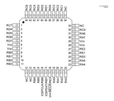
Figure 6. 44-pin QFN
