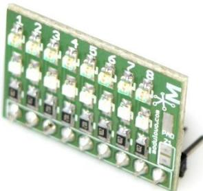
This module enables visual checking of the states on microcontroller leads or integrated circuit leads. In addition, in a simple and visual way you can check bit operations, such as logical shifts (left and right shifts), sum, product and so on.
