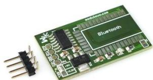
The adapter designed for Bluetooth/UART's module, provides adequate power supply, adjust the voltage levels of UART serial transmission.
