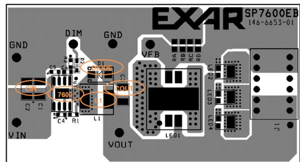
Fig. 18: XRP7603 Eval Board Component Side Lay
