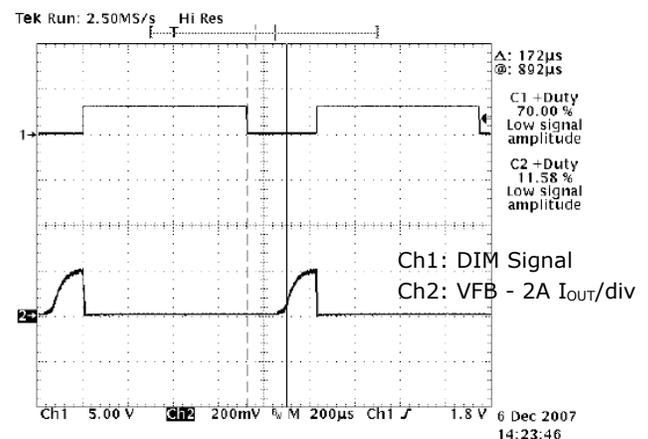
Fig. 15: 1KHz, 70% Duty Cycle
