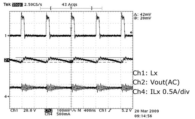
Fig. 9: Cout=1uF, Output Ripple=42mVpp, Vin=29V
