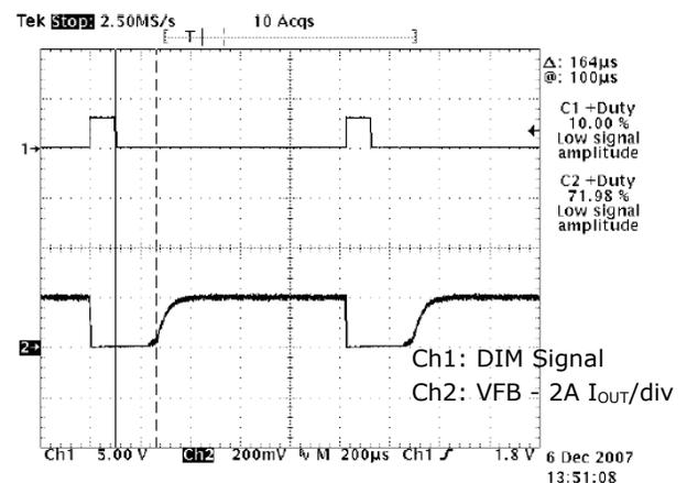
Fig. 14: 1.1KHz, 10% Duty Cycle Dimming Signal
