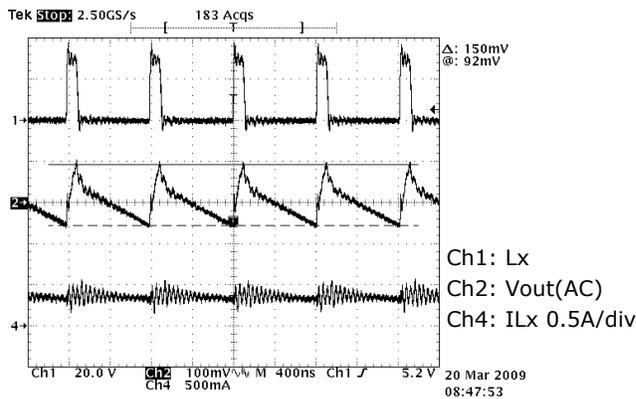
Fig. 8: No Cout, Output Ripple=150mVpp, Vin=29V
