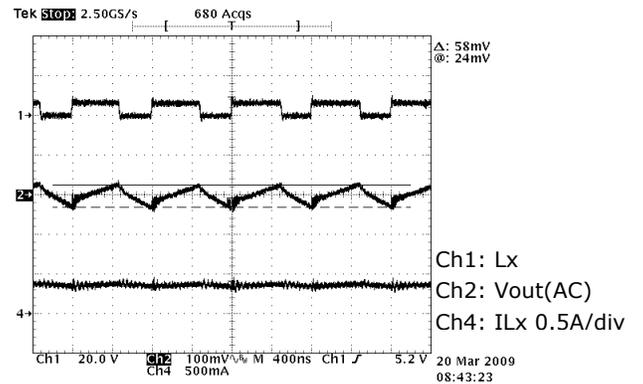
Fig. 7: No Cout, Output Ripple=58mVpp, Vin=6V
