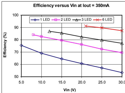
Fig. 4: Efficiency vs Input Voltage
