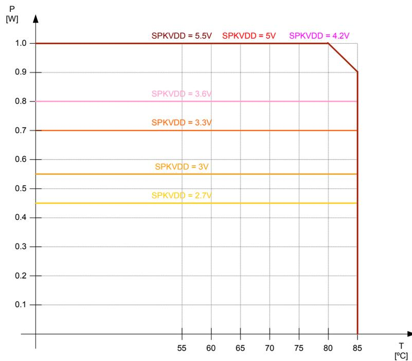
Figure 2 Class D Speaker Power De-Rating Curve
