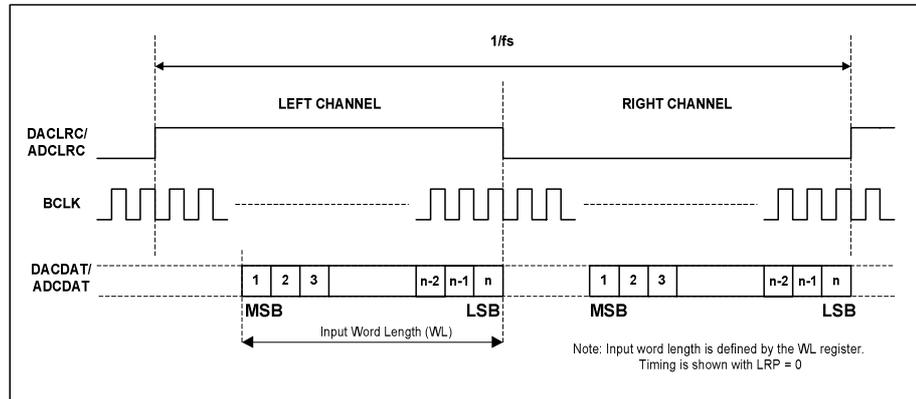
**Figure 66 Right Justified Audio Interface (assuming n-bit word length)**
