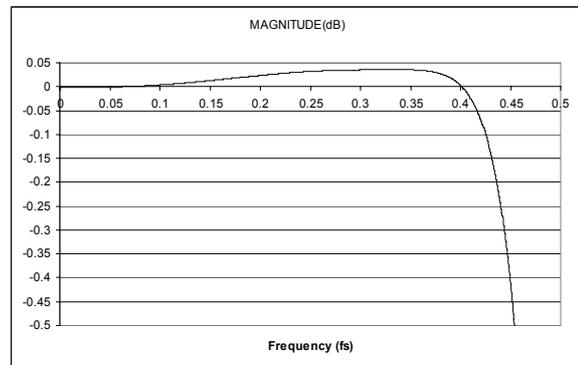
**Figure 97 DAC Digital Filter Ripple (Sloping Stopband Mode)**
