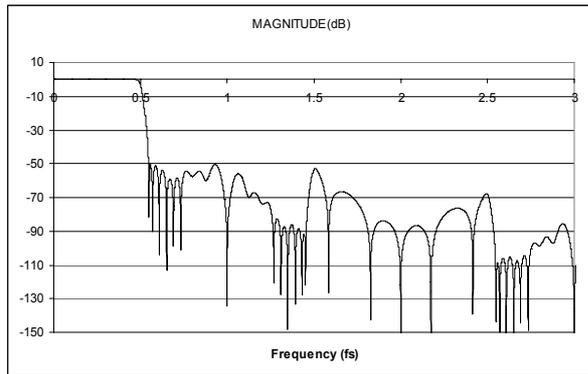
**Figure 94 DAC Digital Filter Frequency Response (Normal Mode)**
