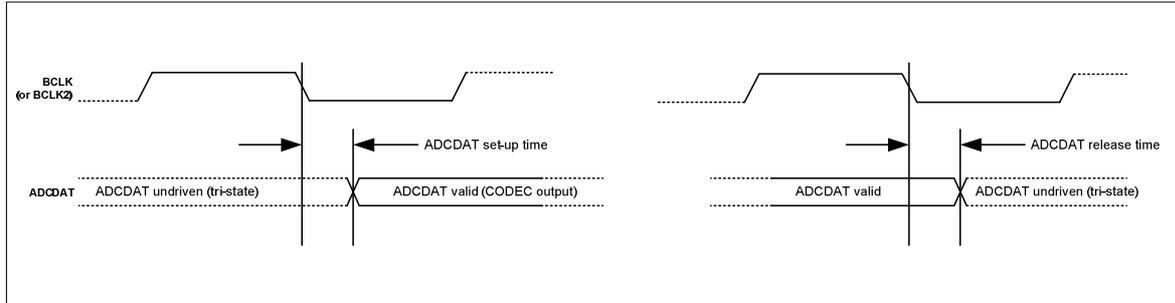
Figure 7 Digital Audio Data Timing - TDM Mode
