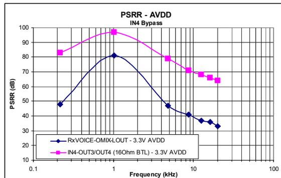
Note: All figures based on 100mVp-p injected on the supply at the relevant test frequency.
