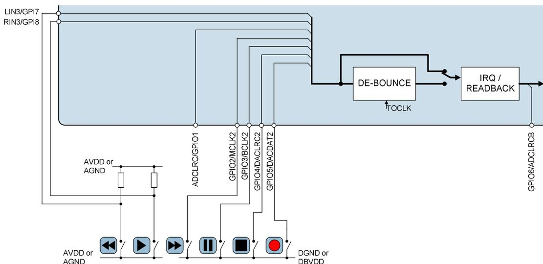
Figure 43 Example of Button Control Using GPIO Pins
