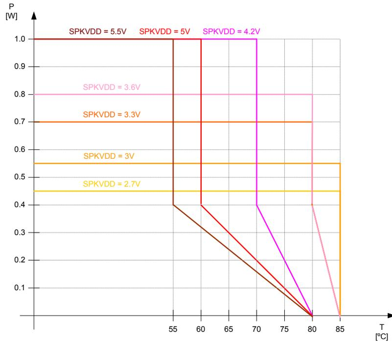
**Figure 3 Class AB Speaker Power De-Rating Curve**
