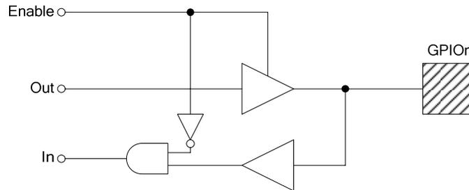
Figure 45 GPIO Pad
