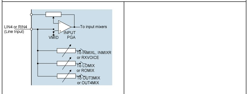
Figure 24 LIN4 or RIN4 as Line Inputs
