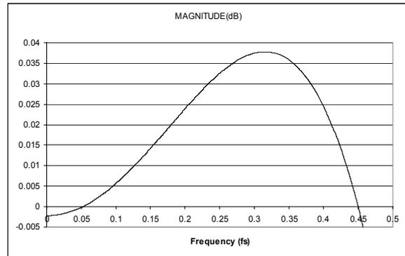
**Figure 95 DAC Digital Filter Ripple (Normal Mode)**
