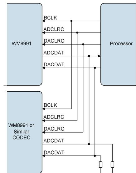
Figure 65 TDM with Processor as Master
