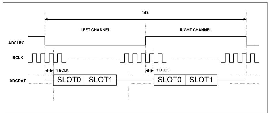
Figure 75 TDM in I<sup>2</sup>S Mode
