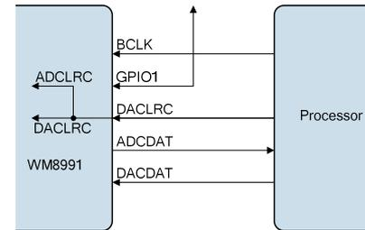
Figure 54 Slave Mode with ADCLRC as GPIO
