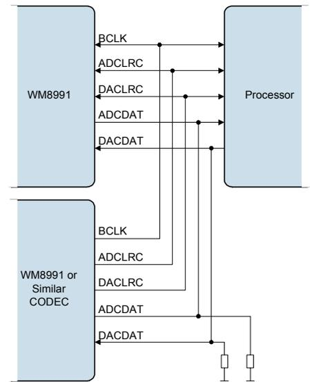
Figure 64 TDM with Other CODEC as Master
