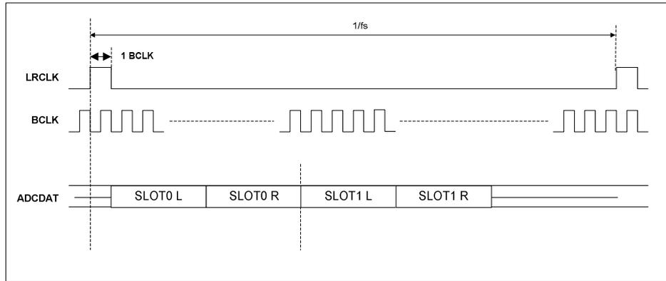
Figure 76 TDM in DSP Mode A
