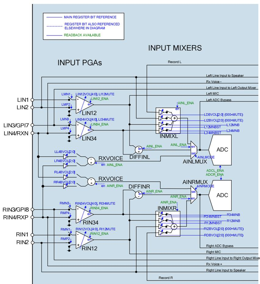
Figure 16 Control Registers for Input Signal Path
