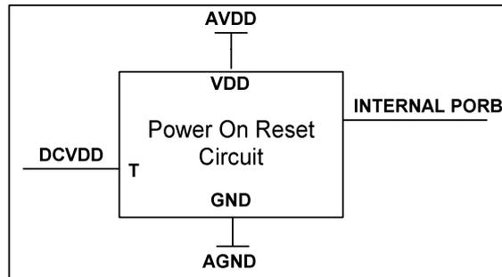
**Figure 13 Internal Power on Reset Circuit Schematic**
