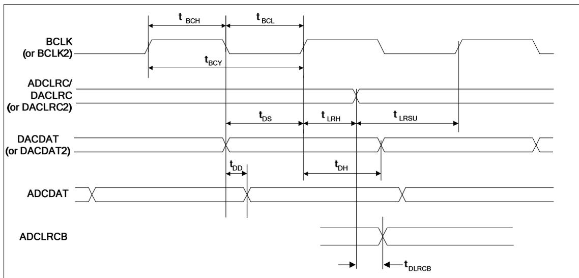
Figure 6 Digital Audio Data Timing – Slave Mode
