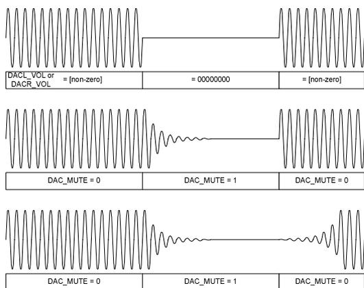
DAC muting and un-muting using volume control bits DACL\_VOL and DACR\_VOL.
