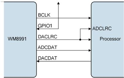
Figure 53 Master Mode with ADCLRC as GPIO
