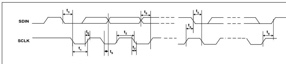
Figure 8 Control Interface Timing – 2-Wire Serial Control Mode
