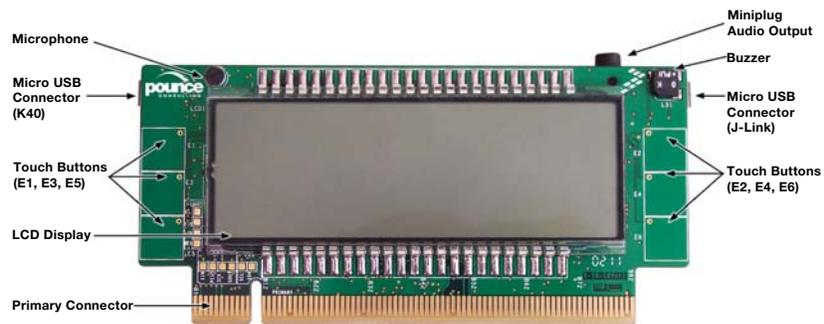
Figure 1: Front Side of KwikStik Development Board
