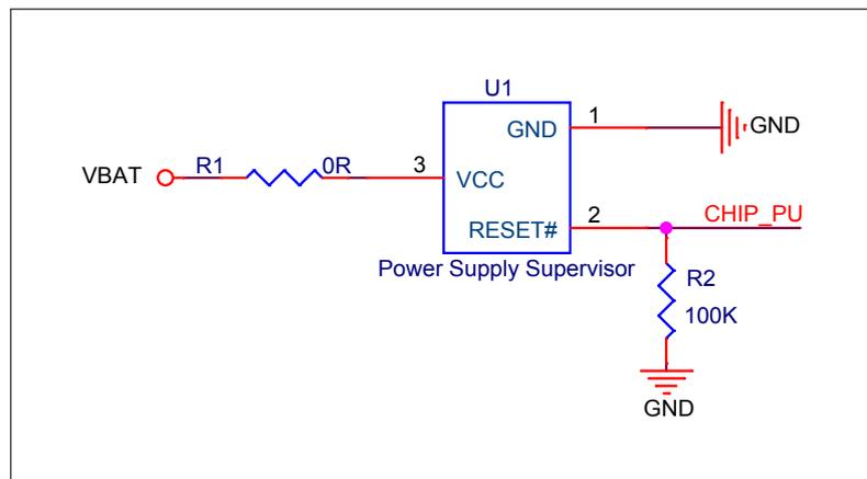
**Figure 6: Reset Circuit****Note:**
