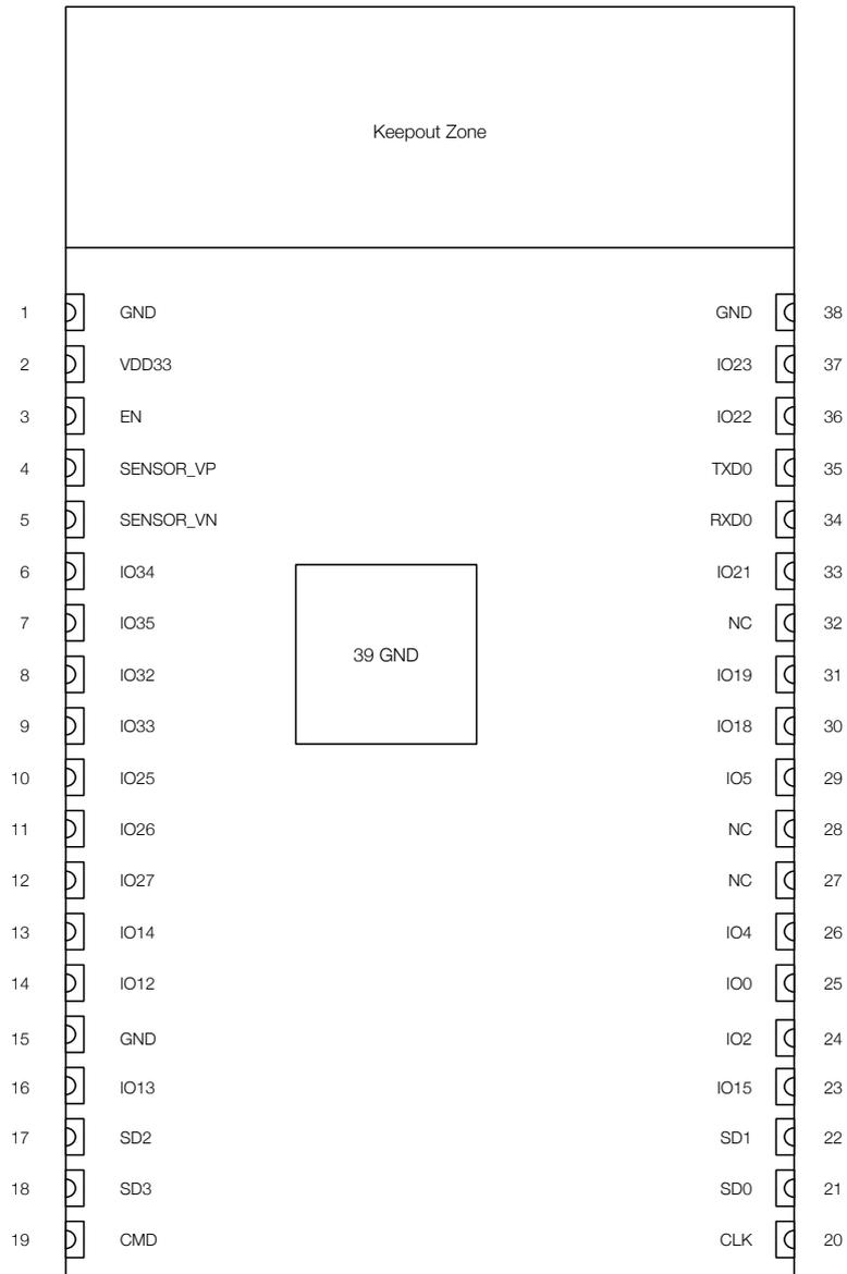
Figure 1: Pin Layout of ESP32-WROVER (Top View)
