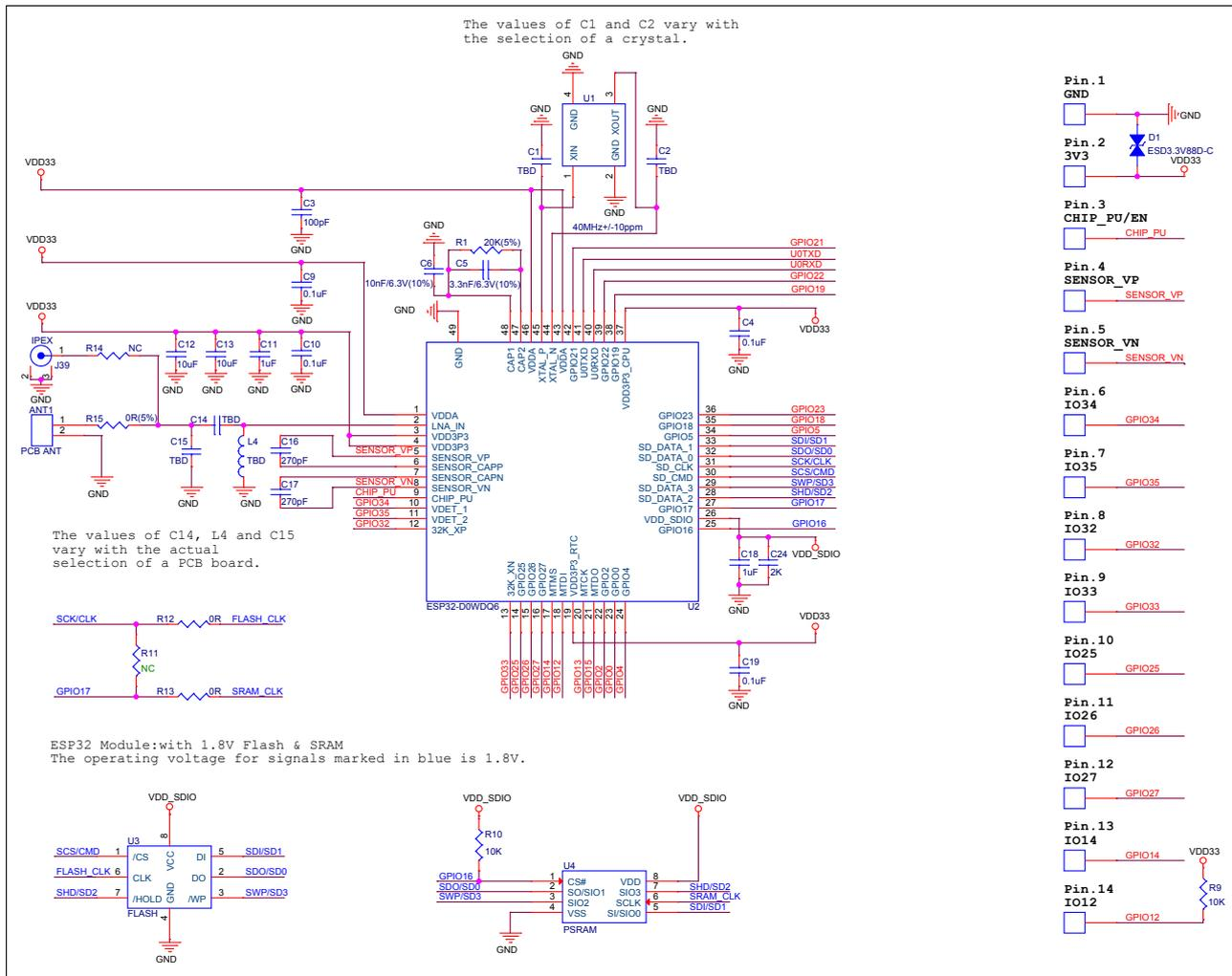
Figure 3: Schematics of ESP32-WROVER
