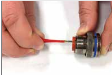
Plastic tool with contact in proper position.
