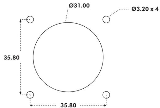
The joystick flange is mounted beneath the panel and the base of the gaiter must be brought through the panel cut-out and held in place with the circular bezel. For panel thicknesses of 3mm, M3 x 16 countersunk machine screws are recommended.
