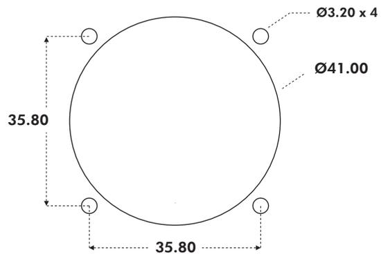
The joystick is dropped into the panel cut-out. For panel thickness of <math>< 3\text{mm}</math>, M3 x 16 countersunk machine screws are recommended.
