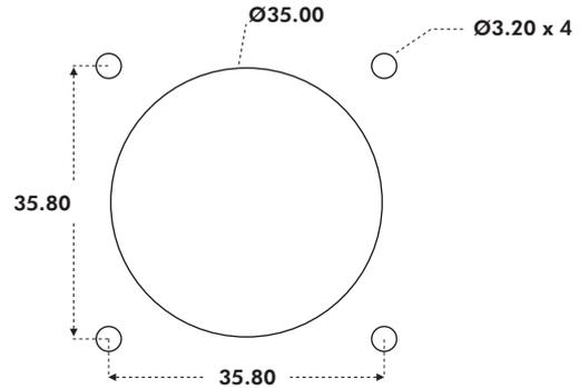
When mounted this way the panel acts as the bezel and no separate bezel is needed. M3 machine screws are recommended.
