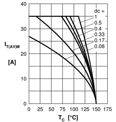
Fig. 6 Max. forward current at case temperature
