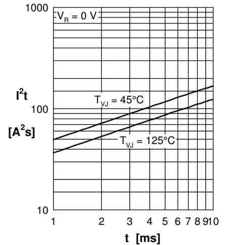
Fig. 3 I<sup>2</sup>t versus time (1-10 ms)
