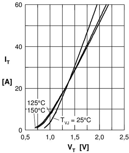
Fig. 1 Forward characteristics
