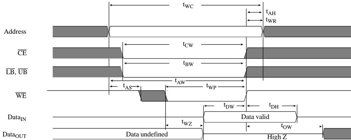
**Write waveform 2 ( $\overline{CE}$  controlled)<sup>10</sup>**
