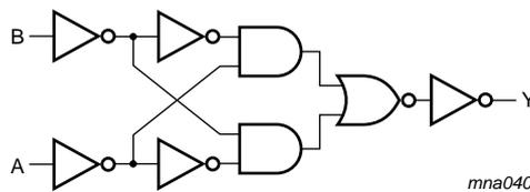
Fig 3. Logic diagram (one gate)
