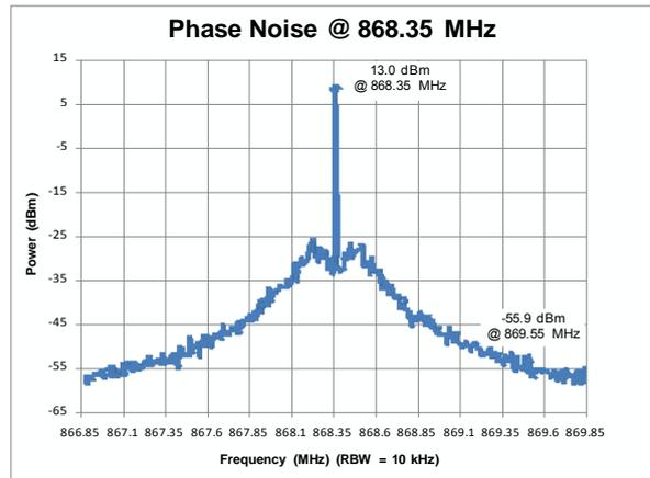
**Figure 4. Phase Noise,  $F_{RF} = 868.35$  MHz,  $P_{OUT} = +13$  dBm, Unmodulated**
