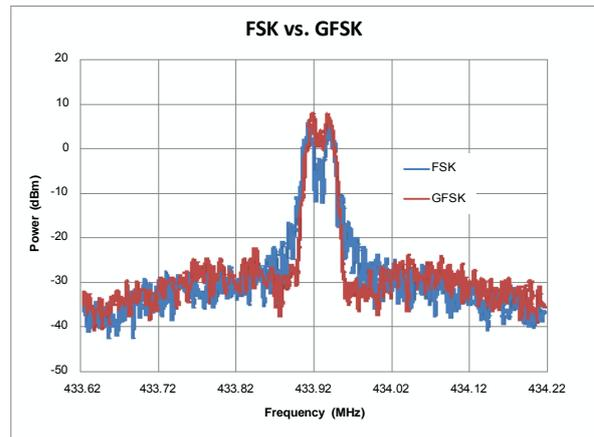
**Figure 6. FSK/GFSK Spectrum, SR = 9.6 kbps,  $F_{DEV} = 15$  kHz**
