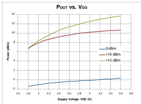
**Figure 8. Output Power vs. Supply Voltages,  $F_{RF} = 433.92$  MHz**
