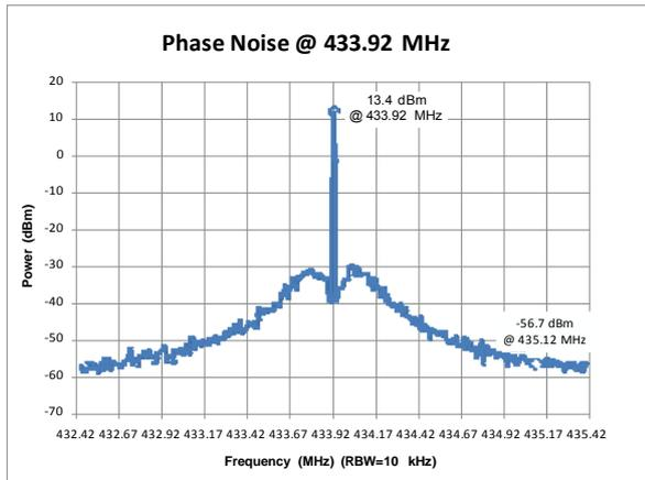
**Figure 3. Phase Noise,  $F_{RF} = 433.92$  MHz,  $P_{OUT} = +13$  dBm, Unmodulated**
