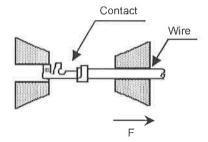
Test method: Pulling load shall be applied between a correctly crimped contact and a wire. The load required to pull the wire out of the contact or break the wire shall be measured. (Testing speed: 25 mm/min.)
