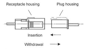
Housing lock shall be removed before the test.
