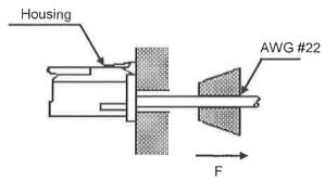
Note) Retainer shall be removed before the test.
