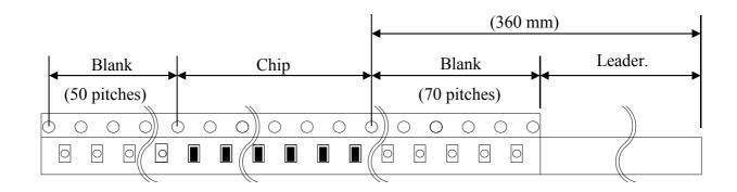
Material of carrier tape : Polystyrene Material of cover tape : Polyester
