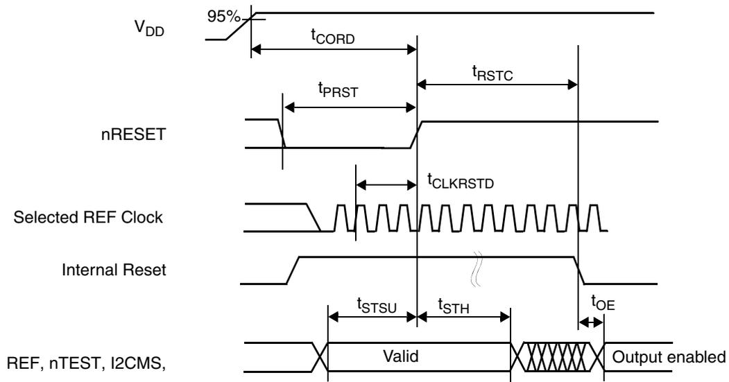
Figure 11. Device Reset
