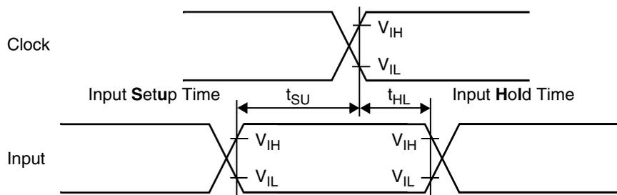
Figure 9. Input Setup and Hold Time
