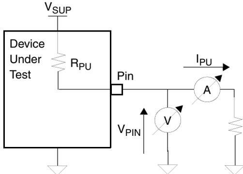
Figure 6. Internal Resistor Test Conditions,  $T_A = 0^{\circ}\text{C}$  to  $70^{\circ}\text{C}$
