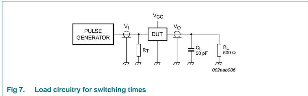
Fig 7. Load circuitry for switching times
