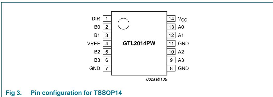
**Fig 3. Pin configuration for TSSOP14**
