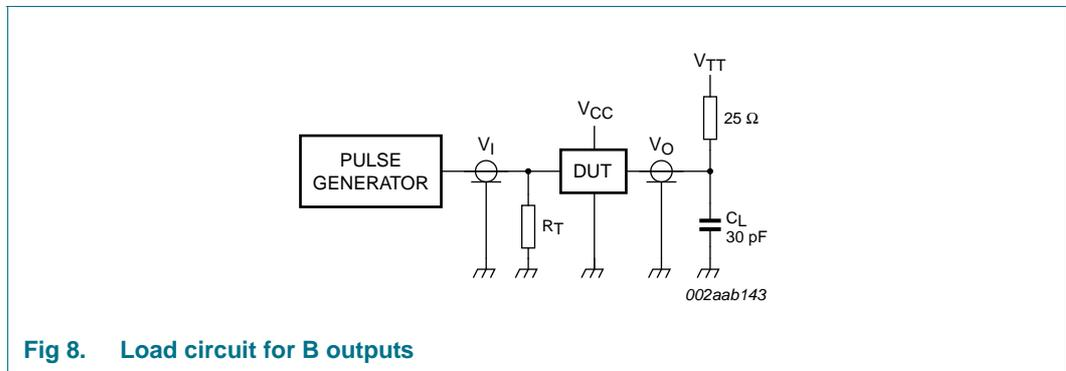
Fig 8. Load circuit for B outputs
