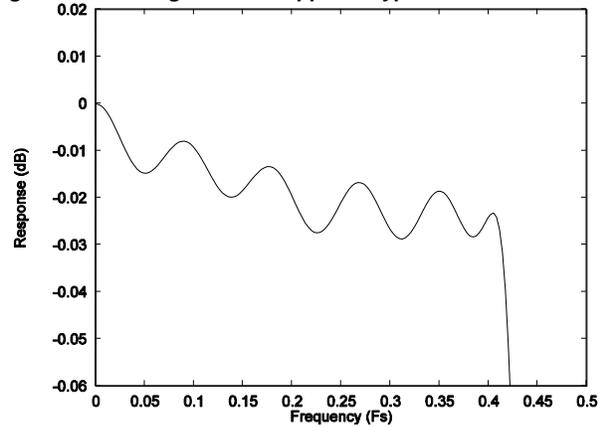
**Figure 32 ADC Digital Filter Ripple – Type 1**
