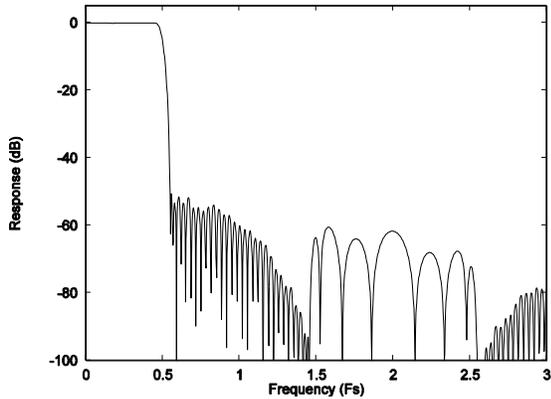
**Figure 23 DAC Digital Filter Frequency Response – Type 1**
