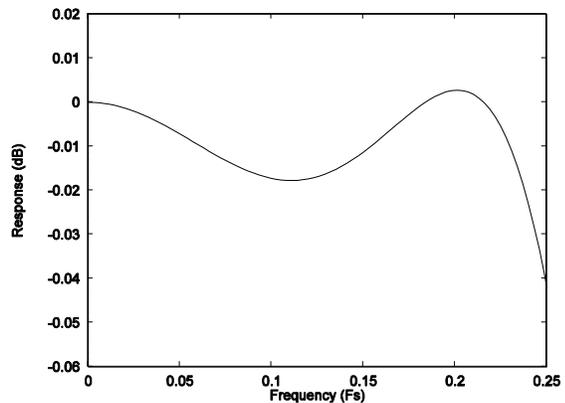
**Figure 26 DAC Digital Filter Ripple – Type 2**
