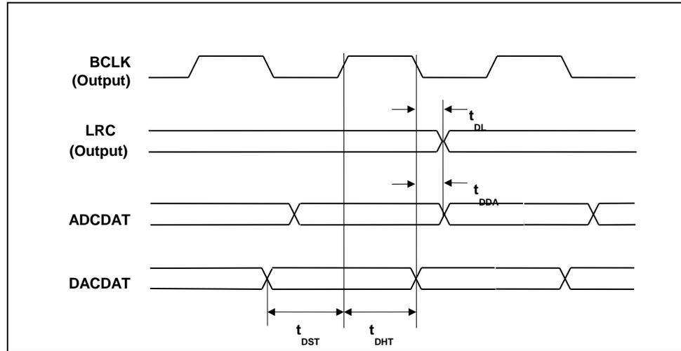
**Figure 2 Digital Audio Data Timing – Master Mode**
