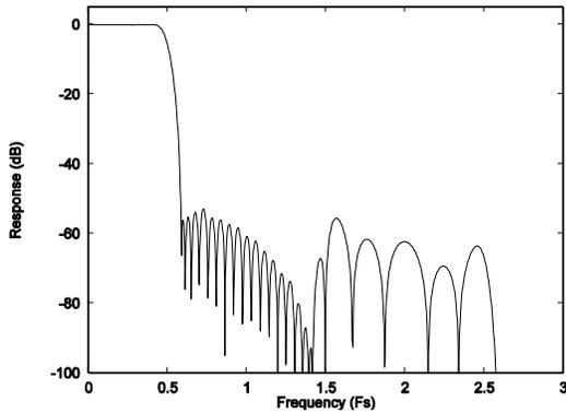
**Figure 21 DAC Digital Filter Frequency Response – Type 0**
