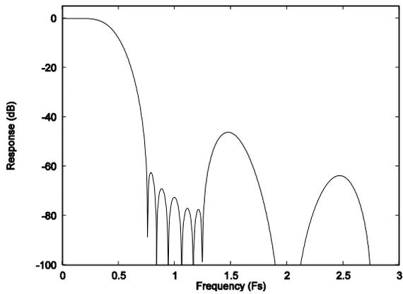
**Figure 33 ADC Digital Filter Frequency Response – Type 2**
