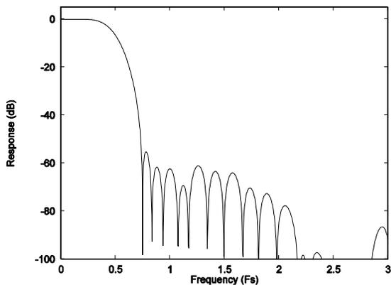
**Figure 25 DAC Digital Filter Frequency Response – Type 2**
