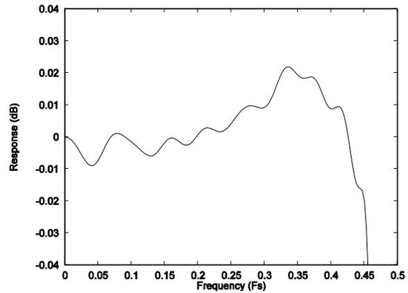
**Figure 30 ADC Digital Filter Ripple – Type 0**
