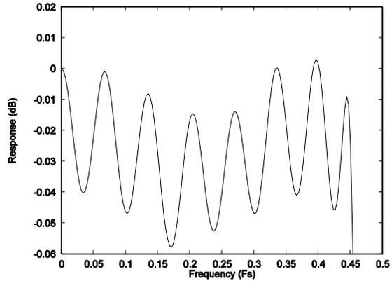
**Figure 24 DAC Digital Filter Ripple – Type 1**
