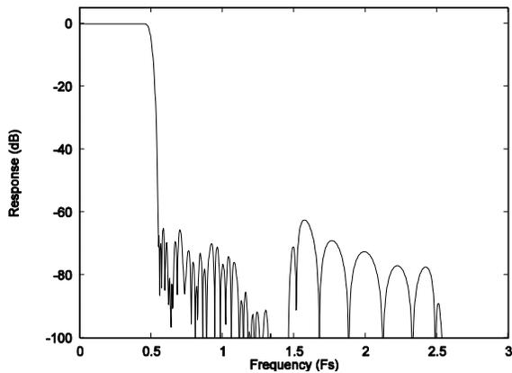
**Figure 29 ADC Digital Filter Frequency Response – Type 0**
