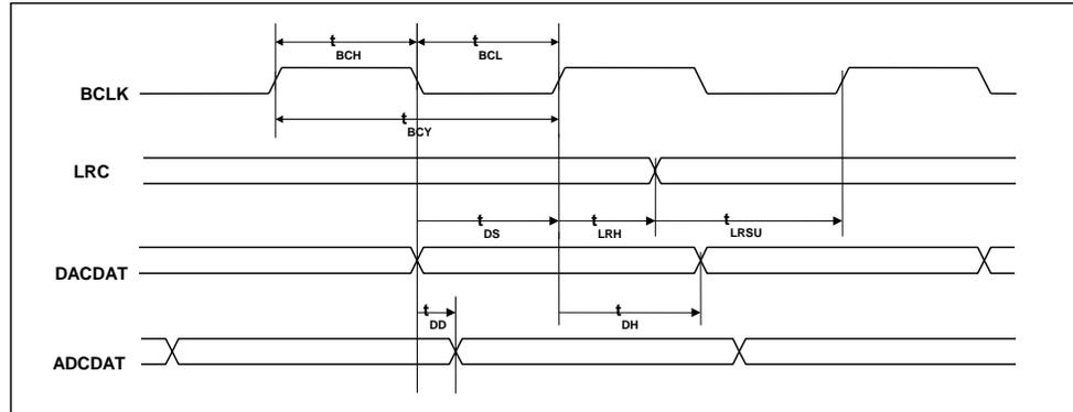
**Figure 3 Digital Audio Data Timing – Slave Mode**
