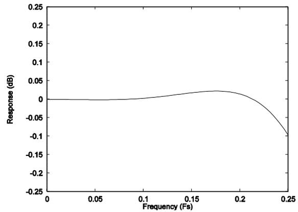
**Figure 36 ADC Digital Filter Ripple – Type 3**
