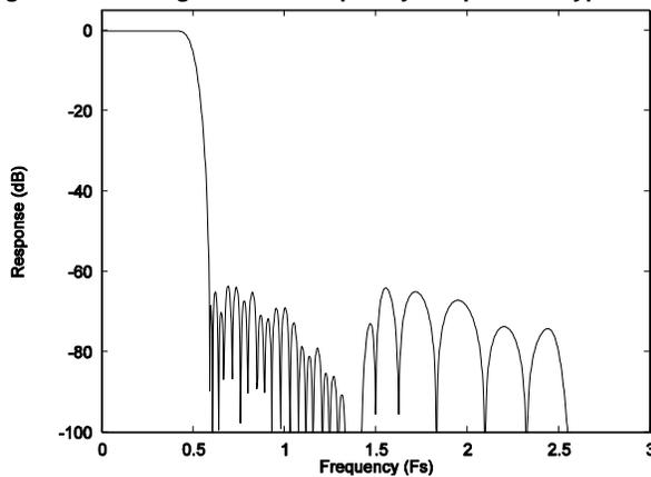
**Figure 31 ADC Digital Filter Frequency Response – Type 1**
