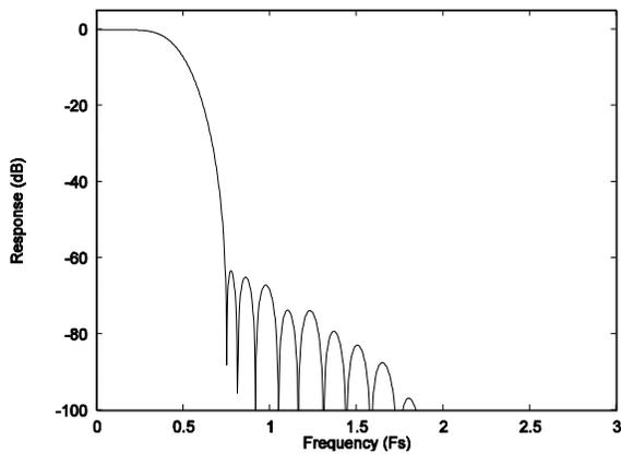
**Figure 35 ADC Digital Filter Frequency Response – Type 2**
