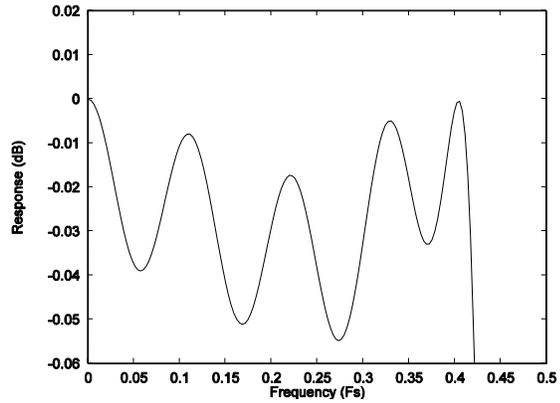
**Figure 22 DAC Digital Filter Ripple – Type 0**
