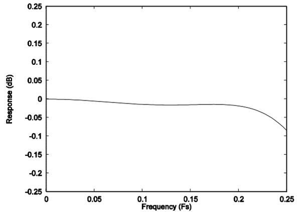
**Figure 34 ADC Digital Filter Ripple – Type 2**
