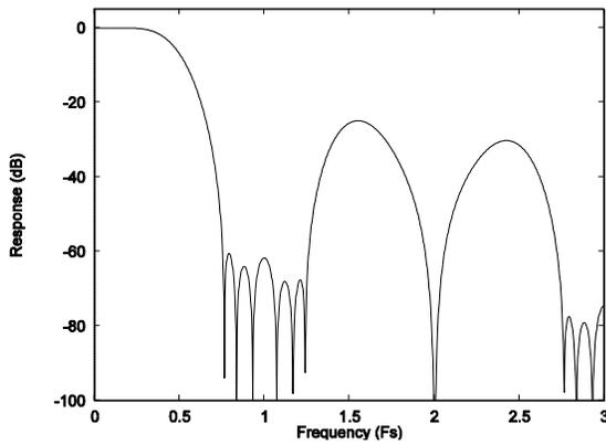
**Figure 27 DAC Digital Filter Frequency Response – Type 3**
