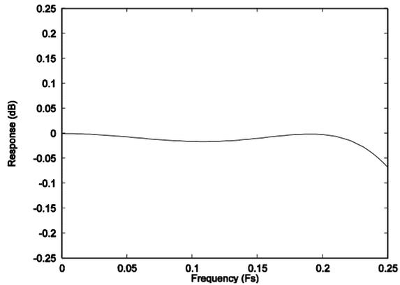
**Figure 28 DAC Digital Filter Ripple – Type 3**
