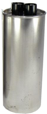
Type HV capacitors are constructed with low loss self healing metallized polypropylene film. Packaged in a cylindrical and oval metal cases. Type HV capacitors are ideal for AC filtering, CVT filtering/snubbing, line current reduction and voltage regulation in power supply applications.
