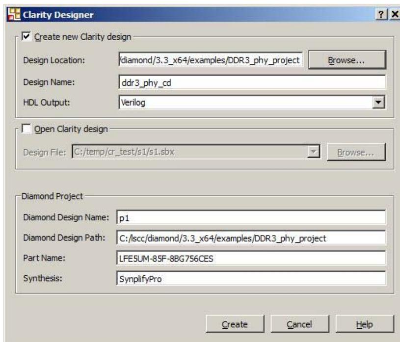
When the **Create** button is clicked, the Clarity Designer IP Catalog window opens as shown in Figure 5-2. You can generate DDR3 PHY IP configuration by double-clicking the IP name in the Catalog tab.
