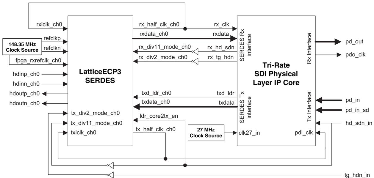
Two sample designs provided with the IP core can be used to implement a complete SDI transmit/receive system on the LatticeECP3 Video Protocol Board. The designs are available in the user's IP project directory after the Tri-Rate SDI PHY IP is generated. A detailed explanation of the sample designs and their usage is provided in the Tri-Rate SDI PHY IP Loopback and Passthrough Sample Designs User's Guide available in the IP project directory.
