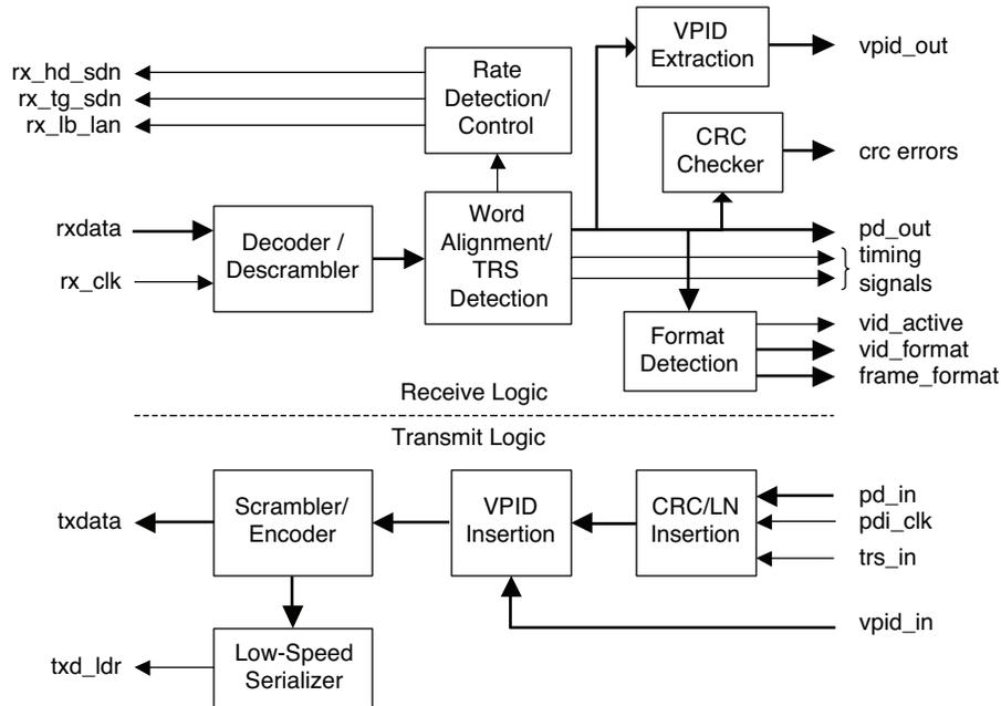
[Figure 2-1](#) shows the top-level functional view of the IP core. As shown, the Tri-Rate SDI PHY IP core does not include the LatticeECP3 SERDES in it. The top portion of the diagram shows the receiver and the bottom portion the transmitter.
