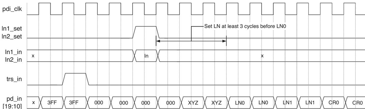
For SD transmission, the trs\_in signal is not used. For HD and 3G-a inputs, trs\_in must coincide with the “3FF” data as shown in [Figure 2-10](#). However, for 3G-b inputs, the trs\_in should go high when the y-channel “3FF” (or the second “3FF”) occurs in the stream as shown in [Figure 2-11](#). The line number for both cases must be set at least three cycles before the LN0 word is given at pd\_in.
