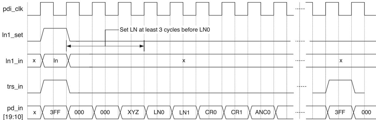
**Figure 2-11. Tx Data and Controls for 3G-b**
