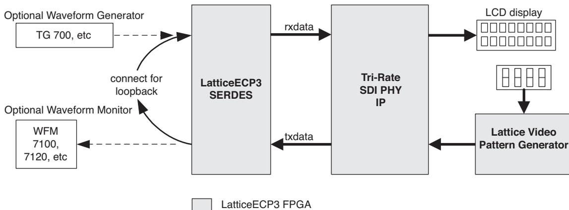
A waveform monitor and/or a waveform generator can be optionally used instead of the loopback cable to monitor and/or source the SDI video. All the transmit functions and most of the receive functions of the IP can be tested with the loopback setup. One major output that is not tested using a loopback cable connection is the actual parallel received data and its relative timing to other status outputs. The passthrough design can be used to test the received video data.
