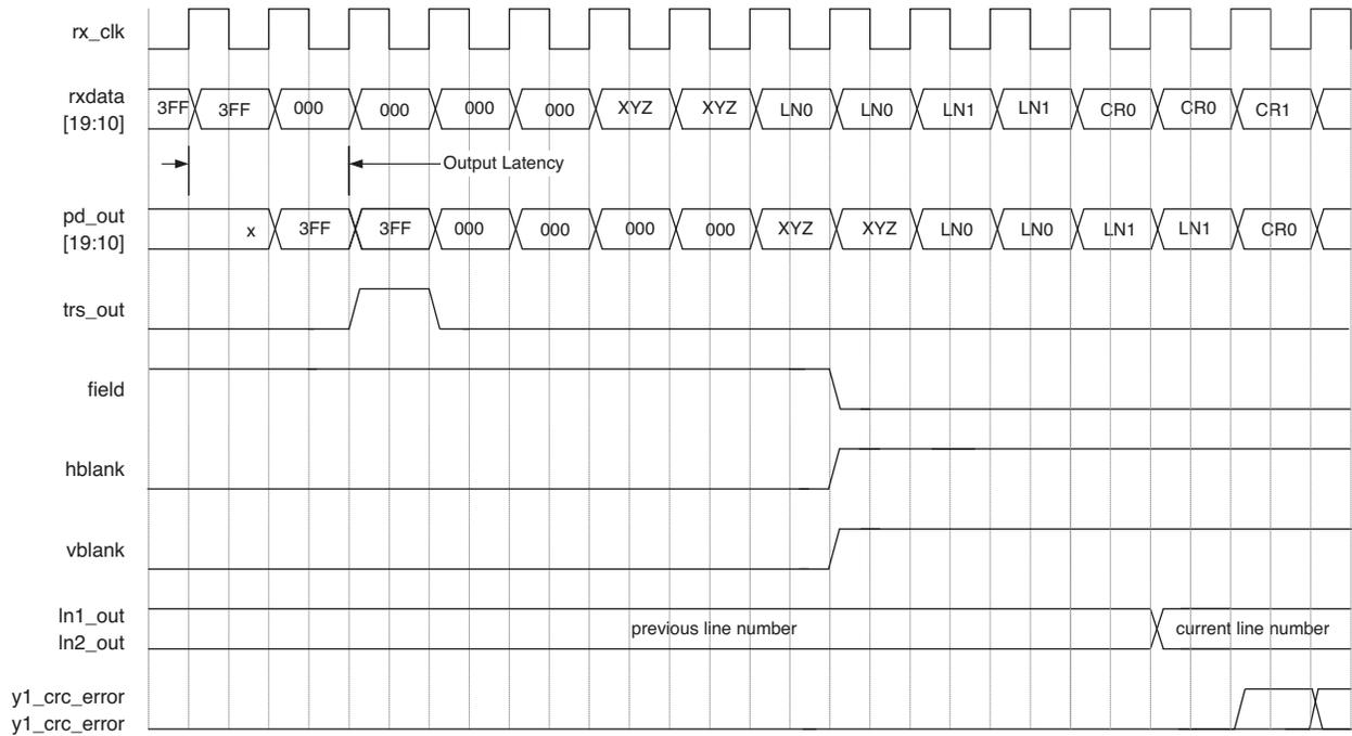
**Figure 2-15. Control Signals for Rx-Side Rate Variations**
