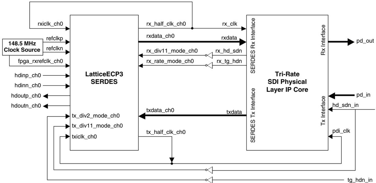
As shown above, one 148.5 MHz clock source is sufficient for multi-rate transmission/reception as long as fractional frame rate HD/3G transmission is not required.
