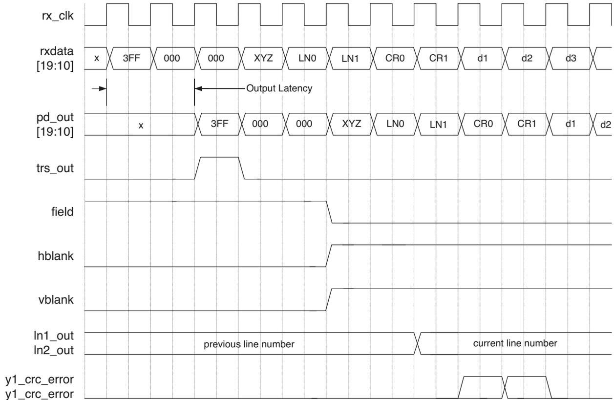
**Figure 2-14. Rx Data and Status Signals for 3G-b**
