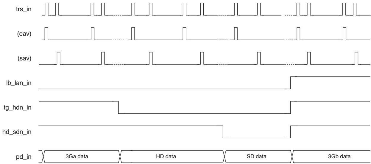
The timing diagram for the Rx side data and status signals for HD/3G-a is shown in [Figure 2-13](#) and that for 3G-b is shown in [Figure 2-14](#). The timing for the multi-rate receive operation is shown in [Figure 2-15](#).
