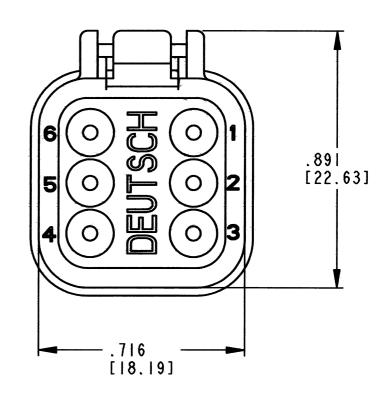
5. SHELL MATERIAL: PLASTIC SEAL MATERIAL: RUBBER
