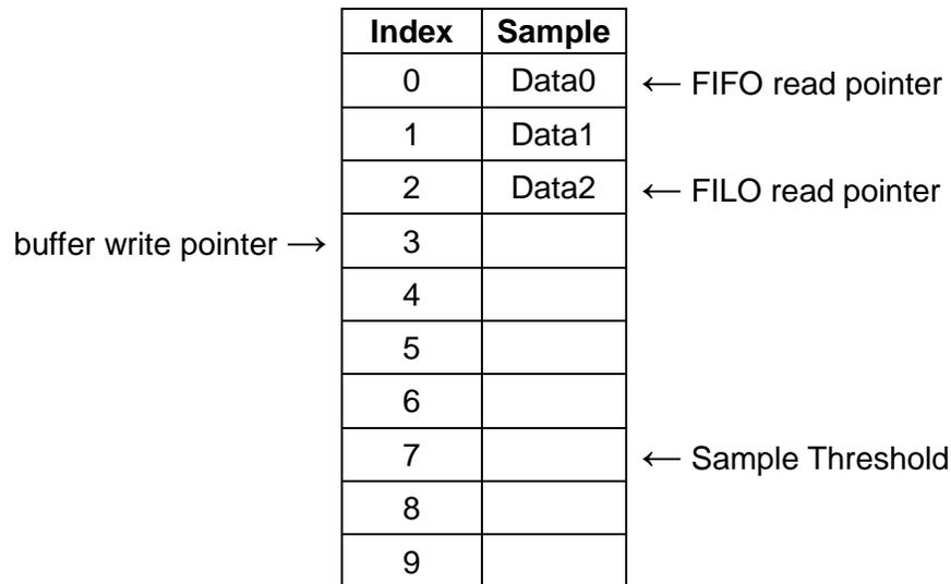
**Figure 17: Buffer Filling**
