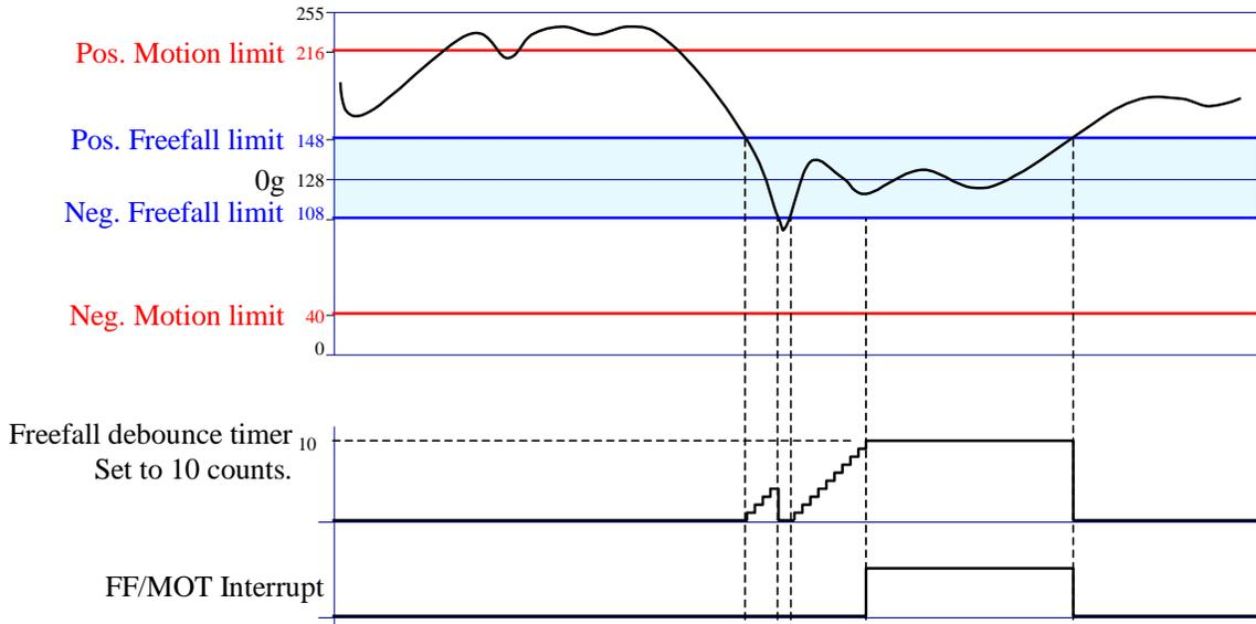
**Figure 14:** Typical Free fall Interrupt Example (FFC ULMODE = 1)
