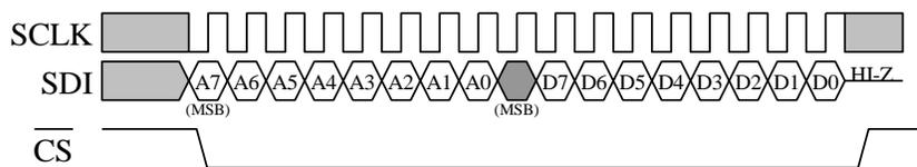
**Figure 7:** Timing Diagram for 8-Bit Register Read Operation
