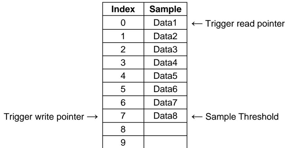
**Figure 20:** Additional Data Prior to Trigger Event
