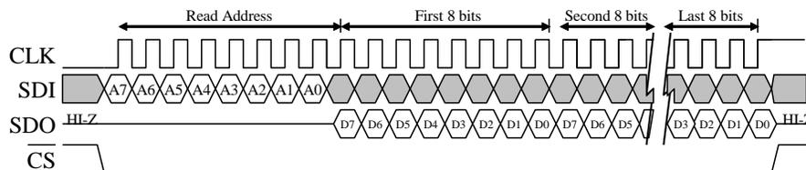
**Figure 4: Timing Diagram for 8-Bit Register Read Operation**
