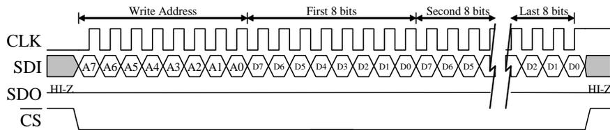
**Figure 3: Timing Diagram for 8-Bit Register Write Operation**
