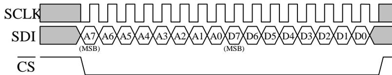
**Figure 6:** Timing Diagram for 8-Bit Register Write Operation
