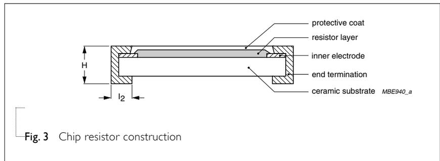
Fig. 3 Chip resistor construction
