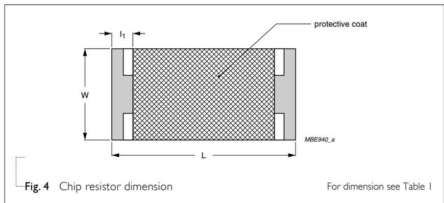
Fig. 4 Chip resistor dimension
