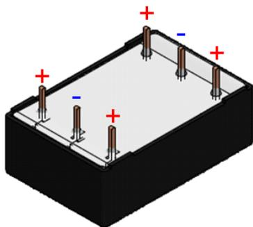
Note that polarity is only for incoming inspection purposes and it does not affect operation. If put under reverse rated voltage  $V_R$ , CeraLink is repoled and works identically.
