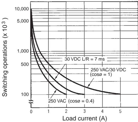
**Reference:** A maximum current of 0.15 A can be switched at 125 VDC (cosφ = 1) and a maximum current of 0.1 A can be switched at 125 VDC and L/R = 7ms. In both cases, a life of 100,000 operations can be expected. The minimum applicable load is 10 mA at 5 VDC (failure level: P).
