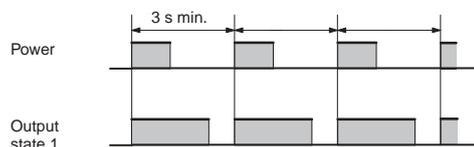
If it is required that the output be turned on repeatedly with an interval of shorter than 3 s, consider using the H3BA-N in mode D (signal OFF-delay).
