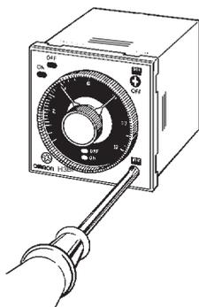
The time required for switching (0.05, 0.1, 0.25, 0.5, 0.75, or 1.0 second) from the star operation to the delta operation of the H3BG-N8/N8H can be selected with the star-delta transfer time selector at the lower right corner of the front panel.
