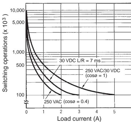
**Reference:** A maximum current of 0.15 A can be switched at 125 VDC (cosφ = 1) and a maximum current of 0.1 A can be switched at 125 VDC and L/R = 7ms. In both cases, a life of 100,000 operations can be expected. The minimum applicable load is 100 mA at 5 VDC (failure level: P).
