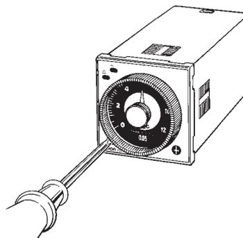
For ON-time, the desired time unit (sec, 10 s, min, and hrs, or 10 s, 10 min, hrs, and 10 h) is indicated in the ON-time unit display window at the lower right corner of the front panel and can be changed by turning the ON-time unit selector located below the ON-time unit display window.
