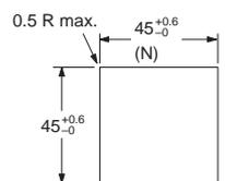
**Dimensions with Flush Mounting Adapter
