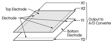
2. To interpret the touched position, 5V is applied to the top electrode (X1 and X2). Then the voltage on the arrow direction evenly changes.
