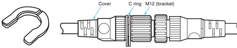
This C ring prevents the M12 connector from becoming loose. When you attach the C ring, press it securely between the bracket and cover.
