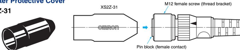
The Sputter Protective Cover protects the connector from weld sputter. Make sure it covers the entire connector.
