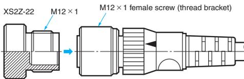
You can use the Water-resistant Cover when the connector is not connected to ensure an IP67 degree of protection. When mounting the Water-resistant Cover to a Connector, be sure to apply a torque range between 0.39 and 0.49 N·m to tighten the Water-resistant Cover.
