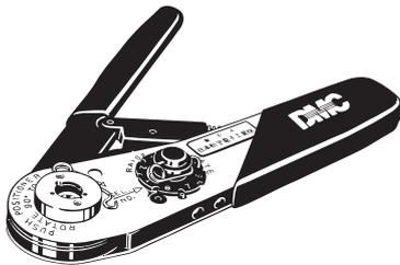
Use the Crimp Tool to crimp a cable core to the XS2U Crimping Pin used with the XS2C or XS2G Crimping Connector.
