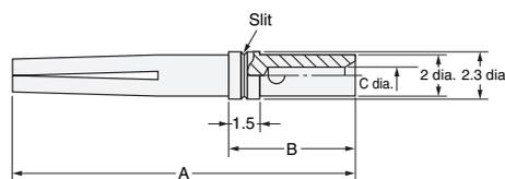
Note: A special tool must be used for crimping. For details, refer to page 24.
