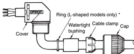
\*A ring is not required for Screw-on Connectors.
