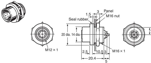
**XS2M-D824-4 Panel-mounting Plug (M12) with Solder Cup Pins and Front Lock**
