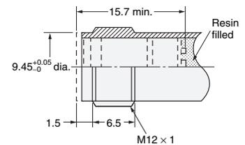
Note: After mounting, anchor the solder cups by injecting resin.
