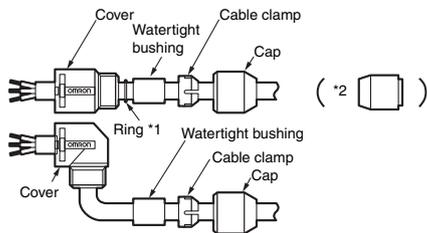
Insulation caps and insulation tubes are included with 5-pole Connectors (XS2C-D5S□ and XS2G-D5S□).
