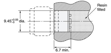
Note: After mounting, anchor the solder cups by injecting resin.
