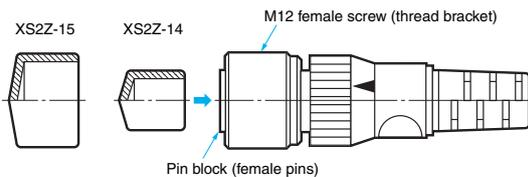
The Dust Cover is for dust prevention and does not ensure IP67 degree of protection. When mounting the Dust Cover to a connector, be sure to press the Dust Cover onto the Connector until the Connector is fully inserted into the Dust Cover.
