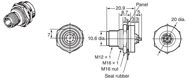
**XS2P-D822-2 Panel-mounting Socket (M12) with Solder Cup Pins and Front Lock**
