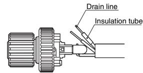
\*When tightening the screws, use the dedicated XW4Z-00B Screwdriver that matches with the screw-slot dimensions.
