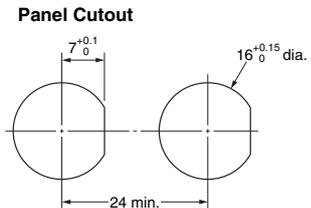
Note: The panel thickness is 1 to 4 mm.
