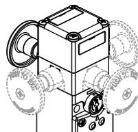
This device is used when the safety switch controls hazardous areas where operators may physically enter with all their body. The release button, oriented towards inside the machinery, allows the exit of the operator accidentally trapped also in case of possible black-out.
