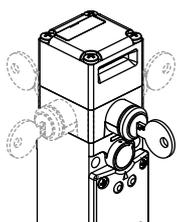
The auxiliary release device with rotating lock is used to allow the maintenance or the entry into the machinery to authorized personnel only. Rotating the key, will make the same action of the solenoid, that is move solenoid contacts and release the actuator. The device can be rotated allowing the installation of the safety switch inside the machinery and
