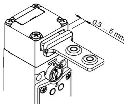
This switch has a wide backlash of the actuator into the head (4,5 mm) to avoid that door gaskets keep in traction the actuator on the solenoid. With closed door, check that the actuator doesn't knock straight against the head of the switch; it must be in the adjustment zone (0,5...5 mm)
