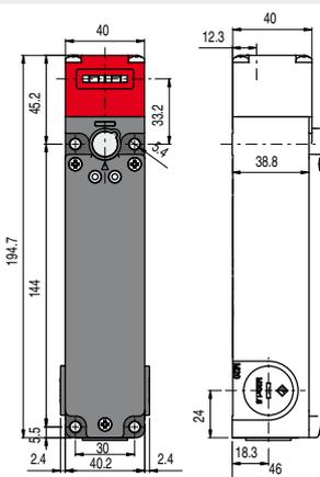
D working principle with lock release device, supplied without actuator
