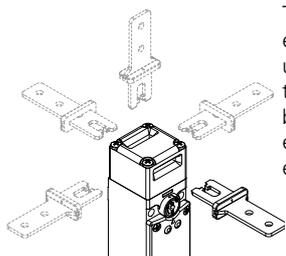
The head can be quickly rotated on each of the 4 sides of the switch by unfastening the four fixing screws. Also the lock release device and the release button can be rotated in 90° steps; this enables the switch to assume 32 different configurations.
