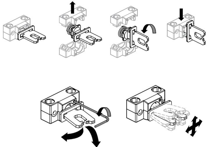
Joined and two directions adjustable actuator for doors with reduced dimensions.
