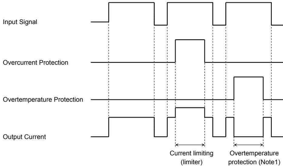
Note1: The overheating detector circuits feature hysteresis. After overheating is detected, normal operation is restored only when the channel temperature falls by the hysteresis amount (5°C typ.) in relation to the overheating detection temperature.
