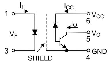
A 0.1- $\mu$ F bypass capacitor must be connected between pins 4 and 6. (See Note 7.)
