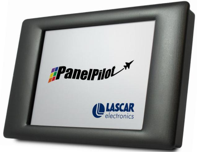
The SGD 28-M is a PanelPilot Compatible graphics display with a 320 x 240 pixel (QVGA) colour display and USB programming interface.
