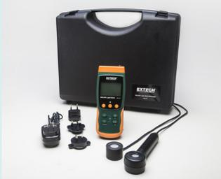
Extech's compact UV Light Meter includes two types of probes: one to measure UVA (long wave 365nm) and the other to measure UVC (short wave 254nm) light sources up to 20mW/cm<sup>2</sup>. The SDL470 date/time stamps and stores files onto an SD card in MS Excel<sup>®</sup> format to make transferring, storing, and analyzing the data on your PC easier. The unit also has a Type K/J thermocouple input to capture temperature readings (temperature probes not included).
