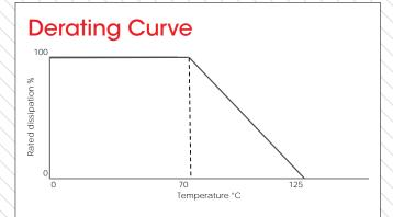
The derated values of dissipation for temperatures in excess of 70°C shall be indicated by the curve above
