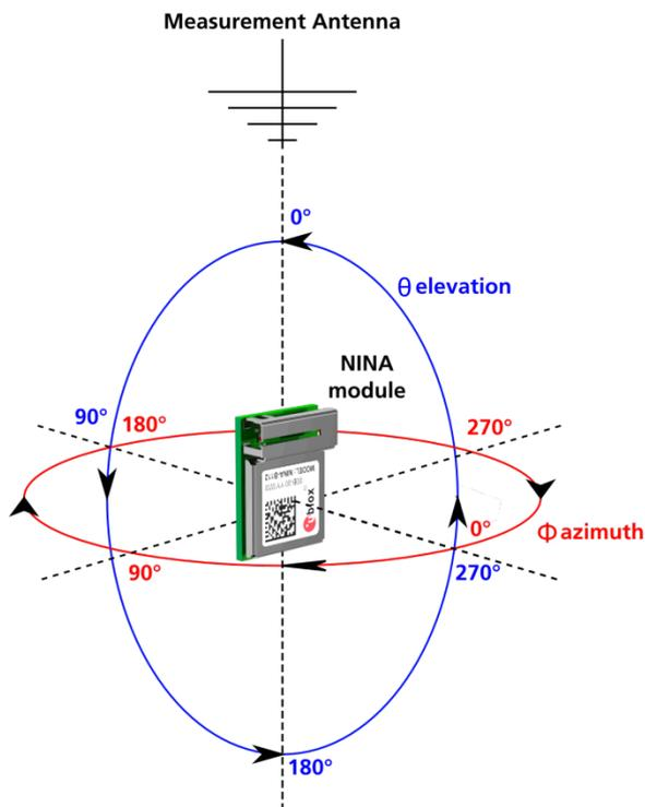
Figure 8: Azimuth and elevation rotation axes relative to the measurement antenna
