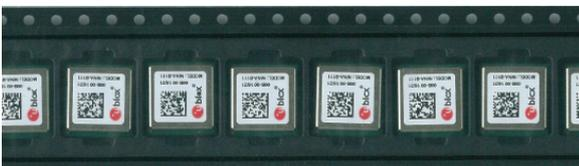
Figure 9: Orientation of NINA-W101 module on tape
