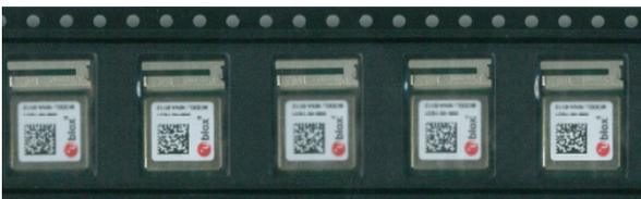
Figure 10: Orientation of NINA-W102 module on tape
