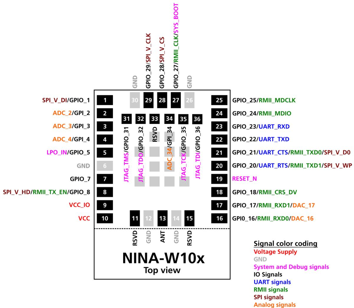
Figure 2: NINA-W10 pin assignment (top view)
